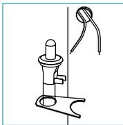
1. Snap switch into mounting plate.
