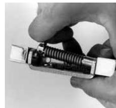
3. Grasping adjustment pin, compress spring and place adjustment bushing assembly over round pin.
