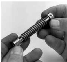
1. Assemble spring cartridge as shown.
