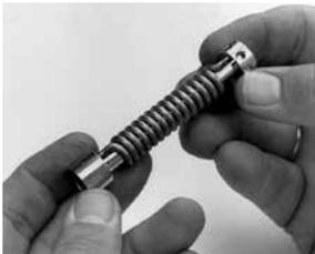
1. Assemble spring cartridge as shown.
