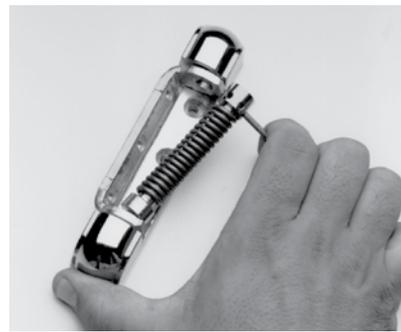
2. Place through washer and bushing over hexagon pin on mounted hinge. Insert adjustment pin into adjustment bushing assembly. Grasping adjustment pin, compress spring and place adjustment bushing assembly over round pin.
